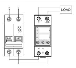
Rated operating current of circuit breaker is 75% maximum current of the relay
